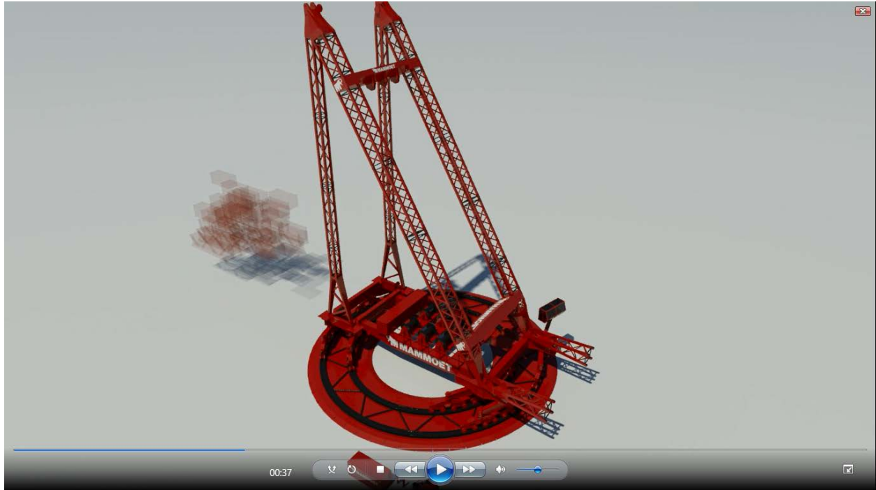
18. Upending backmast with erection spreader.
