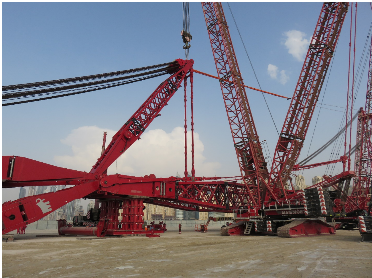
Installing pendant rope and reeving hoist ropes 160914
