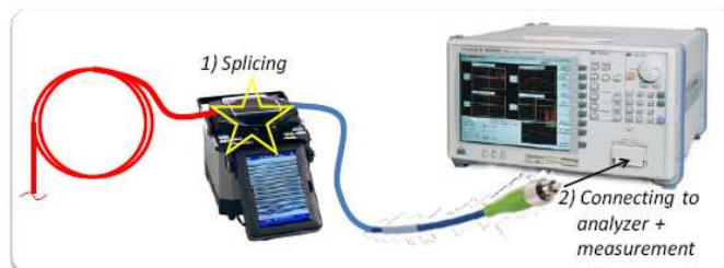
Fig. 5. Splicing of Fibre Optic Cables and Connection to an analyser
